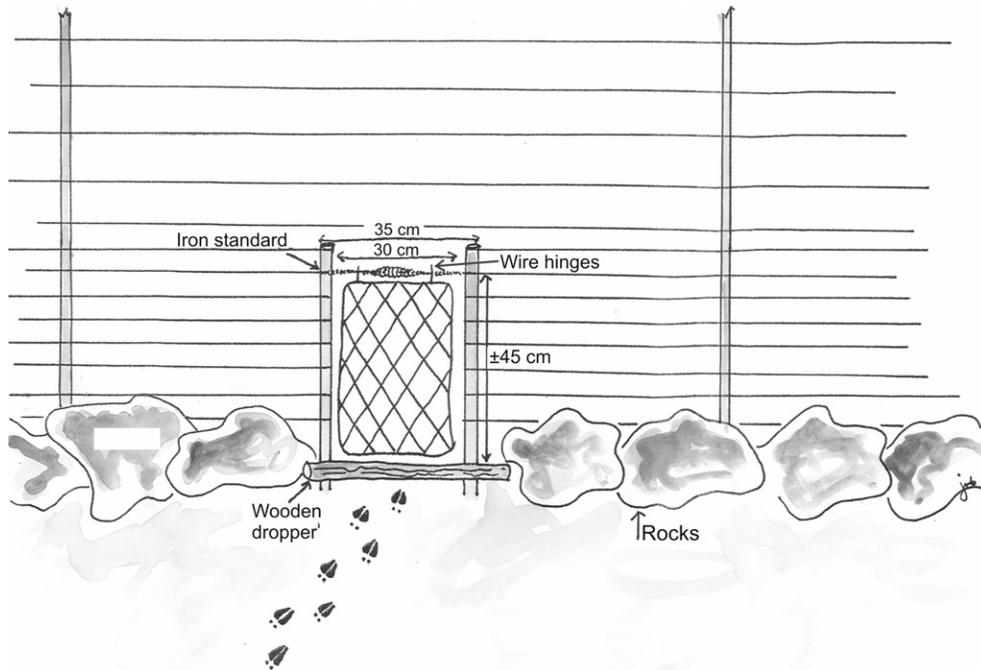
**Fig. 1.** Swing gate design: the gate swings freely on the wire hinges when an animal passes through.
